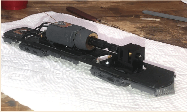
Bowser drive installed onto floor with one-sided PC board cemented to motor and 0.025 wire soldered to it to reach and swipe trolley pole bushing!
